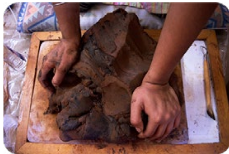
The terracotta is mixed with 10% ash to improve the porosity after firing. More porous = better evaporative cooling.
